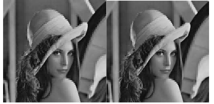
Fig. 3. Reconstructed images using first two level of zero trees. Left: Original EZW Right: Weighted EZW
